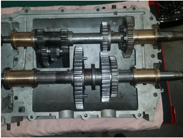
Completed gearbox with new bushes and new gears cit. by the Author
