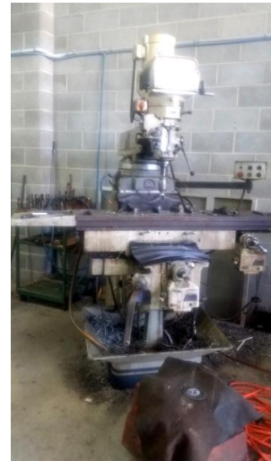
The large Bridgeport type milling machine which was able to handle cutting automotive gears with relative ease
